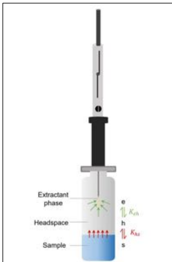
Figure 15. schematic of the three-phase system for SPME. Red is the sample headspace distribution, and green is the headspace extractant phase.
