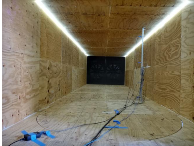
Figure 70. Wind tunnel without screens, honeycombs, spires, roughness elements and baseboard
