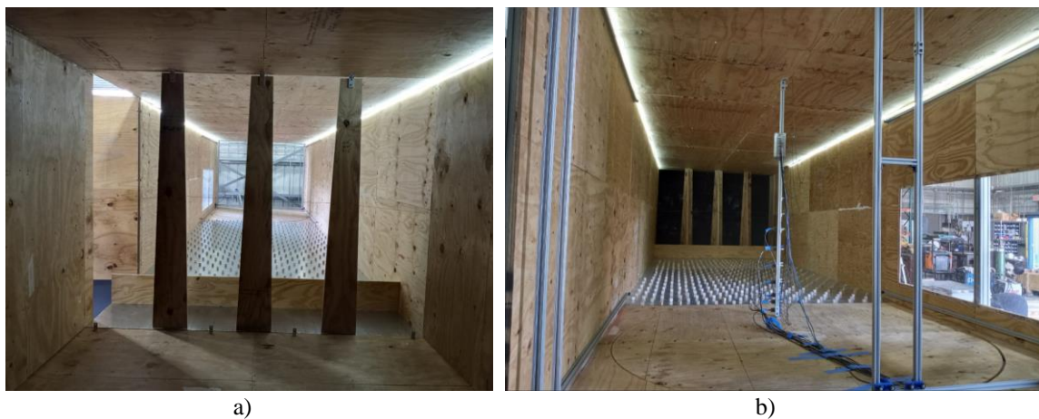
Figure 91. Wind tunnel a) spires and baseboard and b) floor roughness elements
