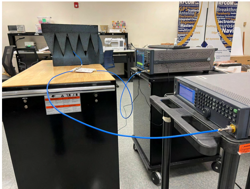
Figure 2.13: Tx-Rx isolation testing with active measurement.
