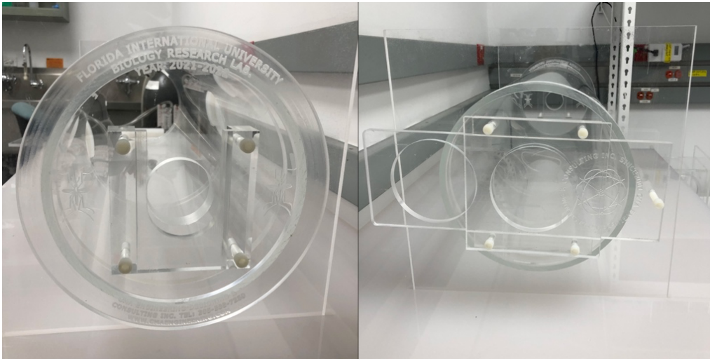
Figure 4. Activated chamber entry (left) and exit plates (right)
