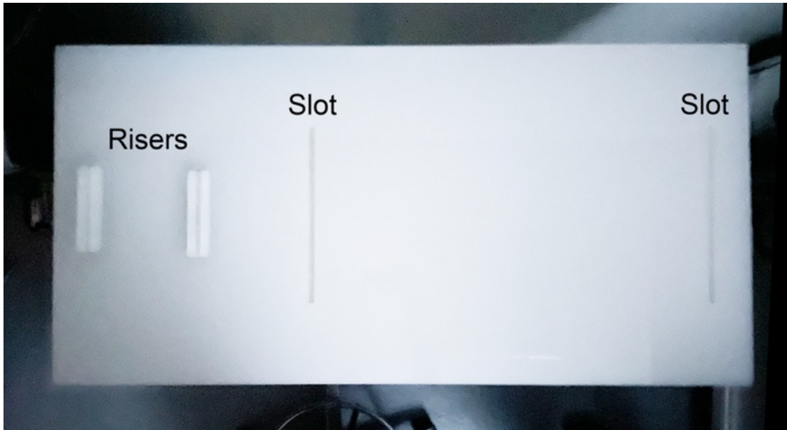
Figure 2. The olfactometer base. The base is made from computer numerical control (CNC) milled white acrylic (24-inch width x 48-inch length x 0.75 inch thick) with 12-inch slots milled to hold the olfactometer component in fixed positions. 6-inch risers hold the stimulus chamber in position but allow for sliding the chamber for easy disassembly. This is designed to hold the olfactometer components securely together, preventing any changes to the olfactometer component alignment to maintain consistency between trials. It is best to bring your olfactometer to the CNC service provider to assure a good fit.
