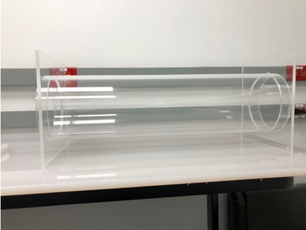
Figure 3. The activated chamber. The chamber is securely fitted to the CNC-milled olfactometer base.
