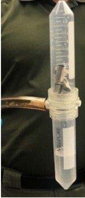
Fig.1.5: Pre-Filter device after attachment and inversion of conical containing casings. Bottom conical contains filtrate with cellular material for step 2. Photo taken at Broward County Sheriff's Office by author.
