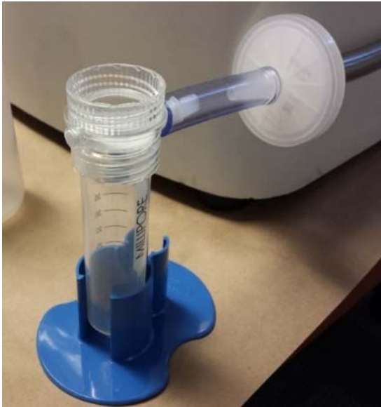
Fig.1.4: Pre-Filter Device with tubing that leads to the vacuum, reproduced with permission from M-Vac Systems, Inc.
