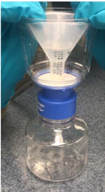
Fig.1.6: Concentration filter using modified funnel insertion for additional concentration of cellular material into smaller diameter area of the filter. Photo taken at Broward County Sheriff's Office by author.
