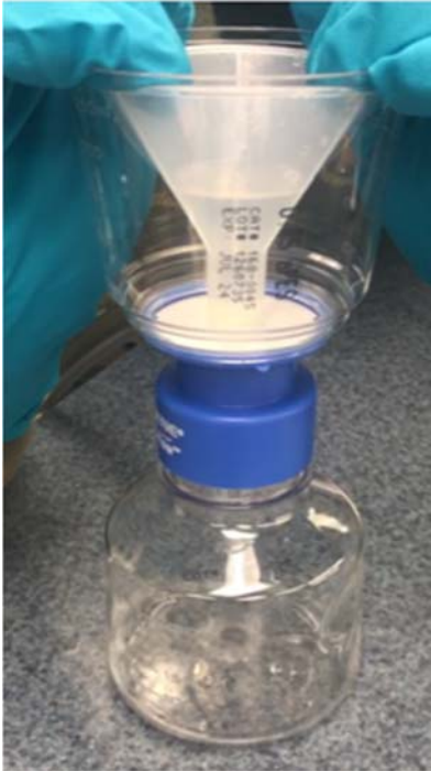
Fig.1.3: Modification to Bardole method with addition of a funnel to concentrate the cells into a smaller diameter portion of the concentration filter. This enables the entire sample to be extracted at one time. Photo taken at Broward Sheriff's Office by author.
