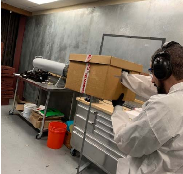
Fig. 1.1: Method for collecting fired cartridge casings, using a cardboard box to catch the FCCs so they did not fall on the ground. Photo taken at Broward County Sheriff's Office by author.
