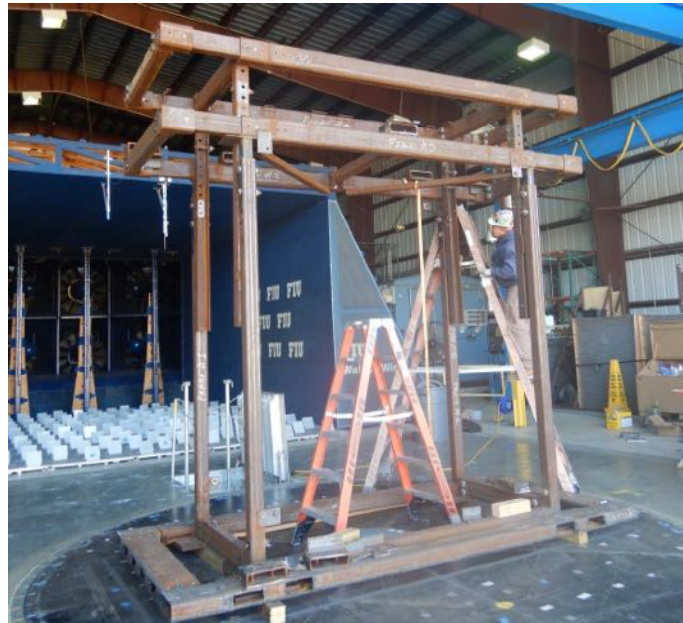
Figure 4.3. Supporting steel structure bolted to the turntable.
