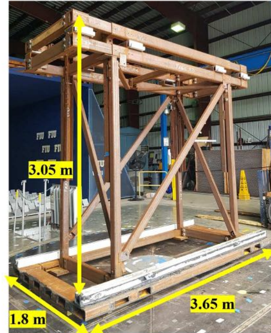
Figure 3.3. Supporting steel structure
