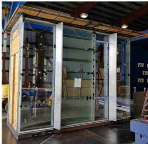
Figure 2.3. Single-skin curtainwall with vertical protrusions: (a) Curtainwall panels; (b) Polycarbonate panels
