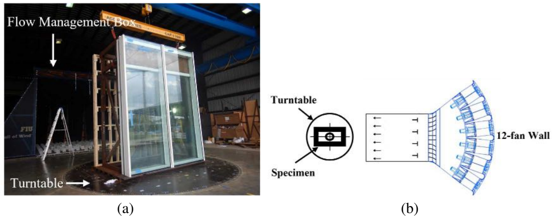
Figure 4.1. FIU Wall of Wind (WOW) Experimental Facility (EF): (a) Inside the WOW EF: Flow management box and the turntable; (b) Schematic drawing of the WOW EF plan
