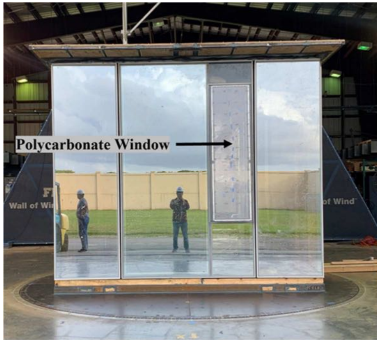
Figure 3.5. Polycarbonate panels and window on the rear side
