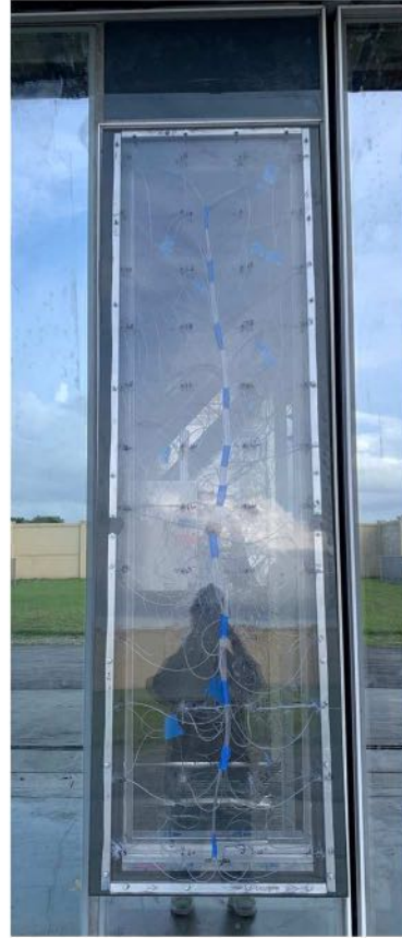
Figure 3.6. Schematic layout of the pressure taps on the polycarbonate side of the operable window system (rear side of the curtainwall)
