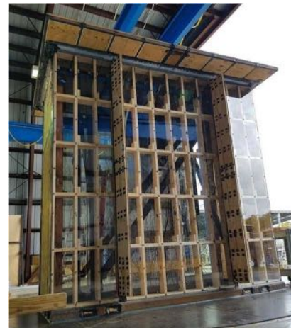
Figure 2.3. Single-skin curtainwall with vertical protrusions: (a) Curtainwall panels; (b) Polycarbonate panels
