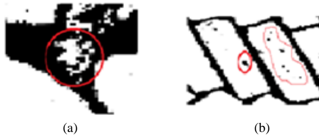
Figure 2.5. Impurities in the binary images: (a) white impurity pixels in mortar (black) and (b) black impurity pixels in bricks (white).
