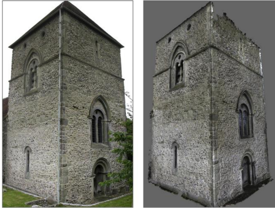
Figure 1.3. A 3D dense point cloud for Jevington Church reconstructed using SfM (Green et al. 2014); Image reused with written permission from the publisher.
