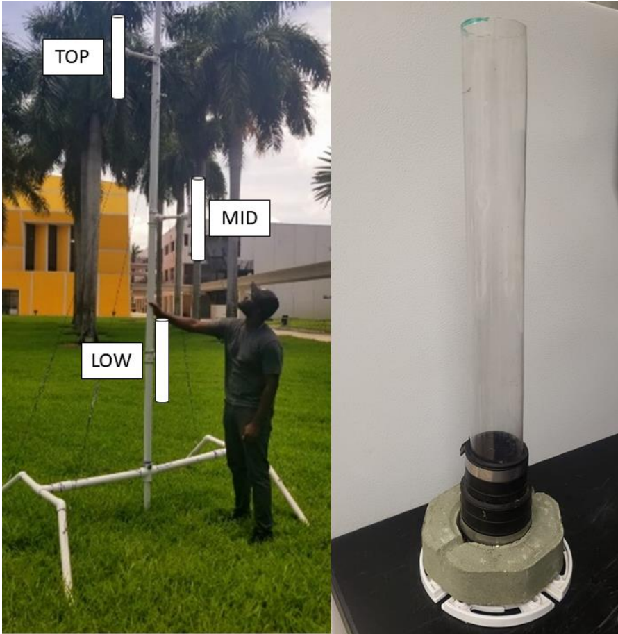
Figure 4.3 a) A photo of a trap tree about 4 m long with 1 m between each trap to collect suspended particulates in the surface mid and low layers in the canal water column. b) a bottom trap deployed near the canal bed with settling particulates. The traps are high aspect ratio (10:1) traps.
