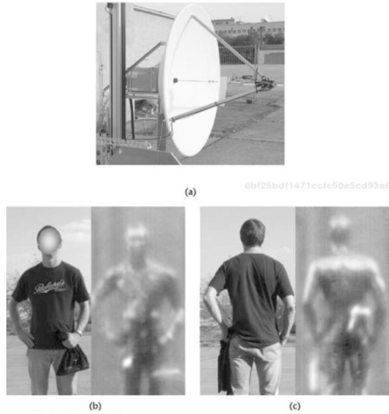
Figure 1-6. (a) 90GHz Radiometric imaging system using a Cassegrain antenna system with a rotating sub-reflector. (b) and (c) radiometer images of a carrying various optically non-visible objects under its clothing. [4].
