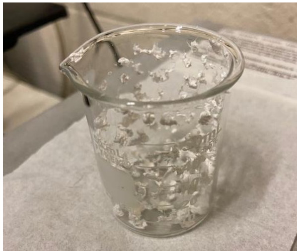
Figure 3.3. Pulled apart BNNTs in a glass beaker before tip sonication.
