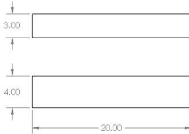
Figure 3.15. DMA specimen dimensions.
