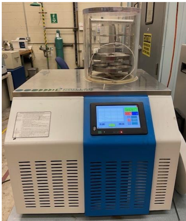
Figure 3.5. Freeze-Dryer showing the sublimation process of BNNP Foams.
