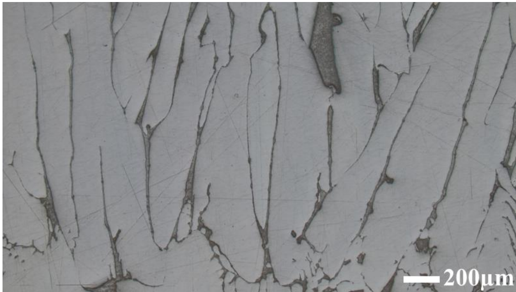
Figure 3.10. Optical image of infiltrated BNNP-cyanate ester composite.
