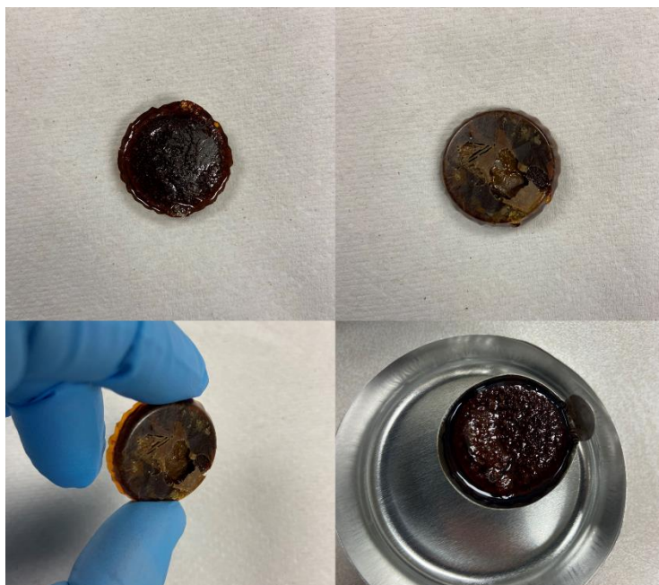
Figure 3.8. Reacted BNNP-CE composite samples after curing.
