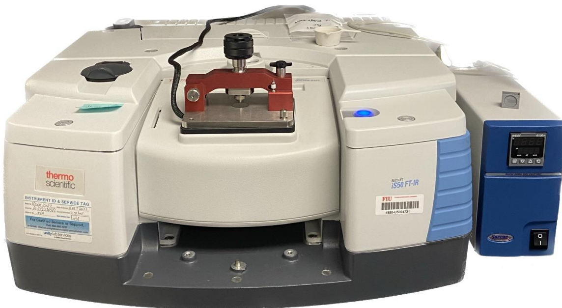
Figure 3.17. The FTIR setup for in situ chemical analysis during curing.
