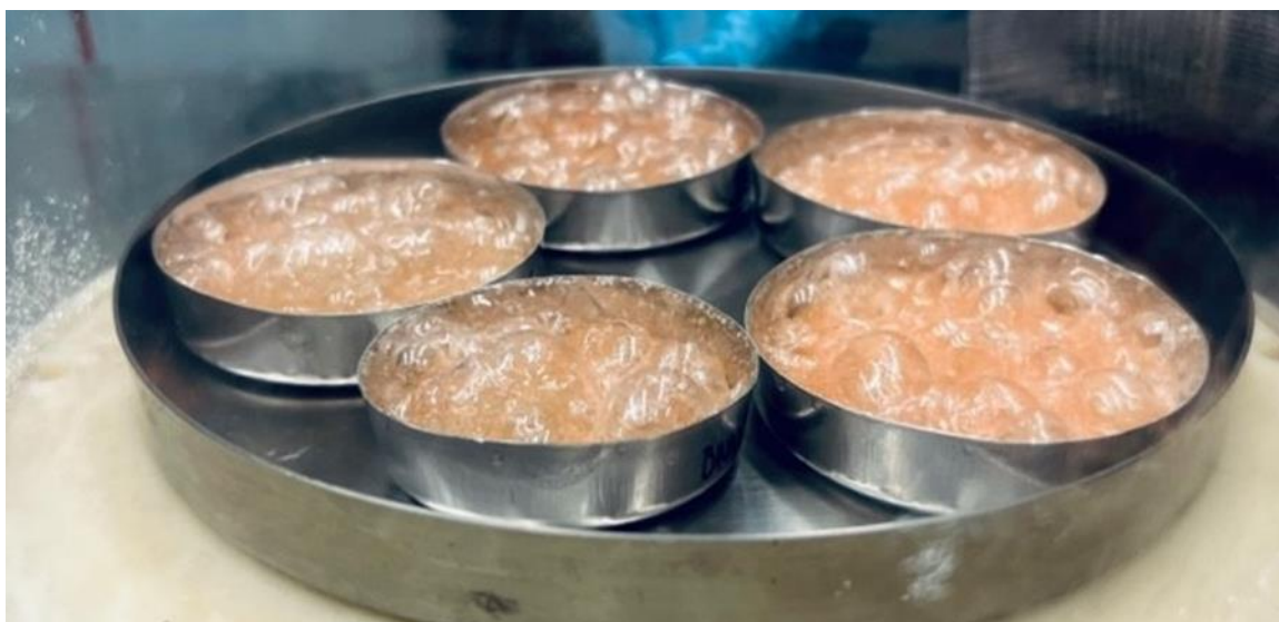
Figure 3.7. BNNP reinforced cyanate ester during the vacuuming process. Both the air trapped in the foam and solvent in the polymer is evaporating
