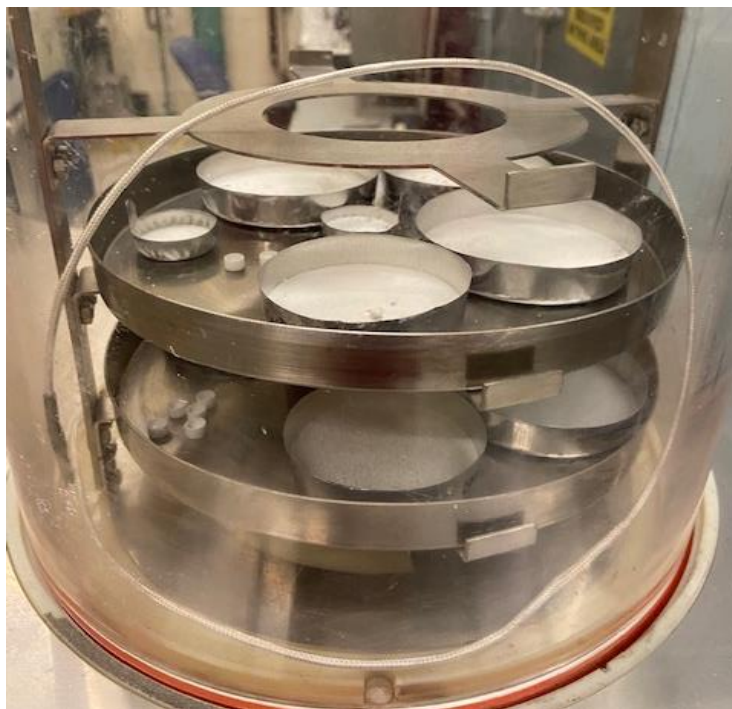
Figure 3.6. BNNP (top rack) and BNNP/BNNT (bottom rack) foams during the sublimation process.
