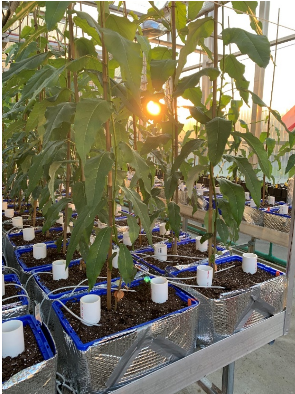
Picture 1: Morning sun graces the greenhouse where P. trichocarpa clones are established for warming treatments. The experimental set up used AKRO grid containers separated into two compartments with a 1-micron mesh and PVC soil respiration collars. The picture was taken on day 44 of the experiment prior to the introduction of clones into temperature treatments. Picture by Chrissi Schnell (DOE ORNL).
