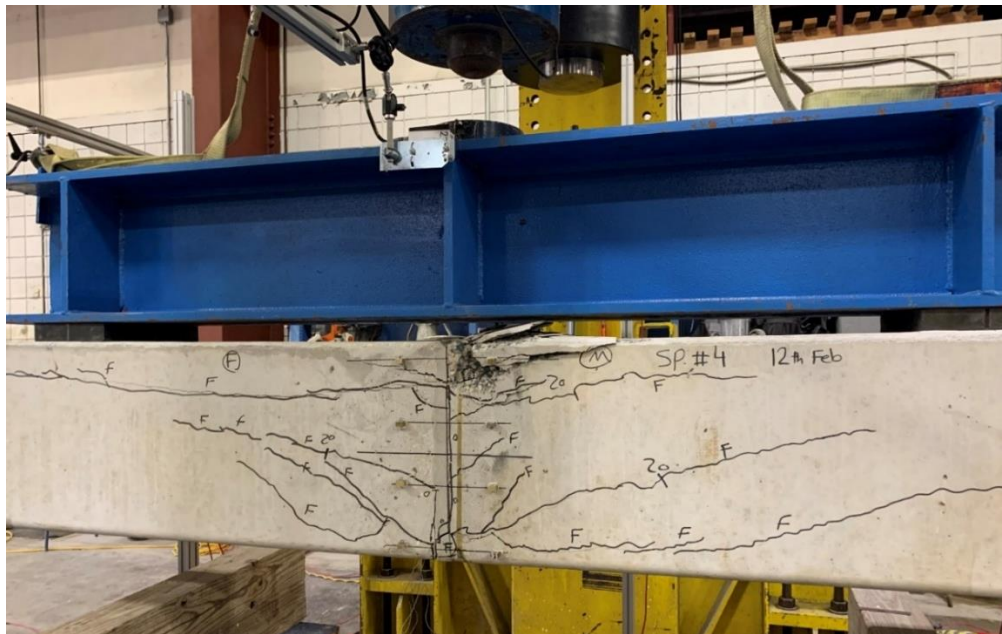
Figure 88: Crack propagation and failure mode of Specimen 4
