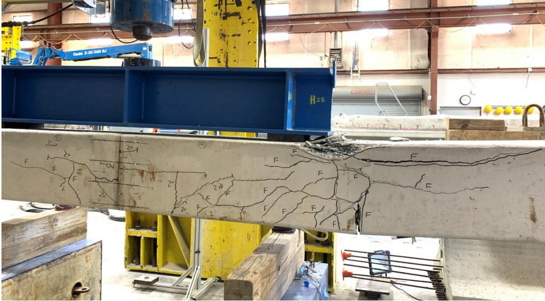
Figure 98: Crack propagation and failure mode of Specimen 6
