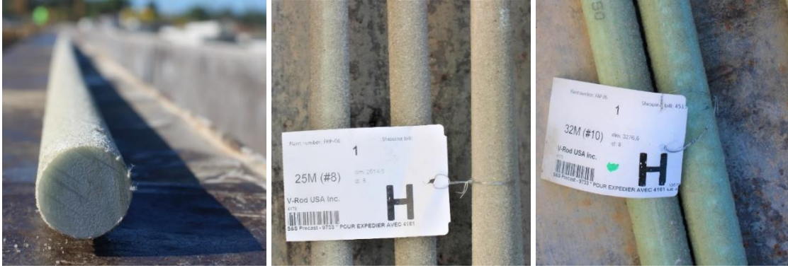
Figure 48: The GFRP bars used for the construction
