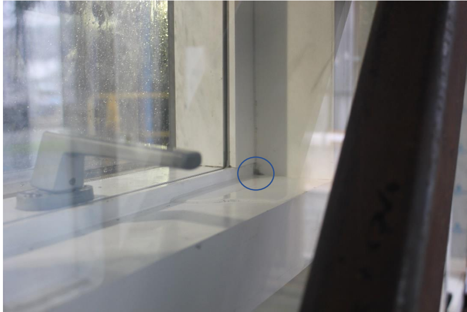
Figure 4.13: Formation of water bubble and deposition of water on the windowsill at 100 mph
