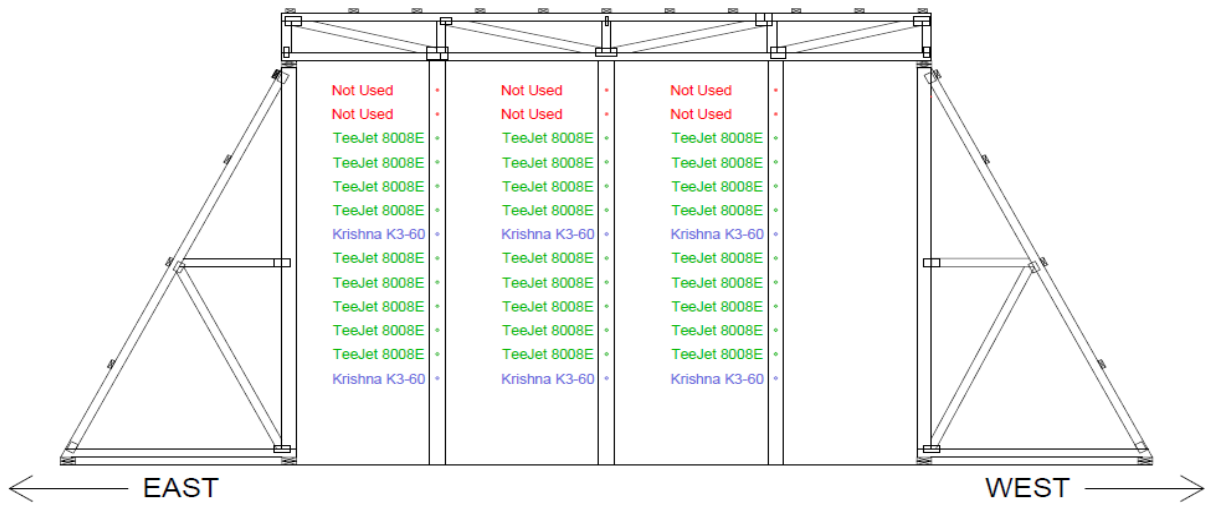
Nozzle Layout for WDR Test #5
