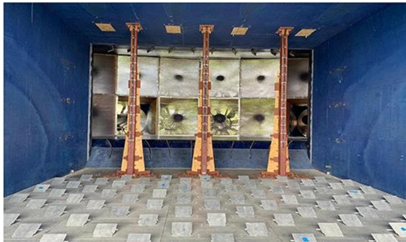
Figure 2.1: Inside flow management box showing roughness elements and spires
