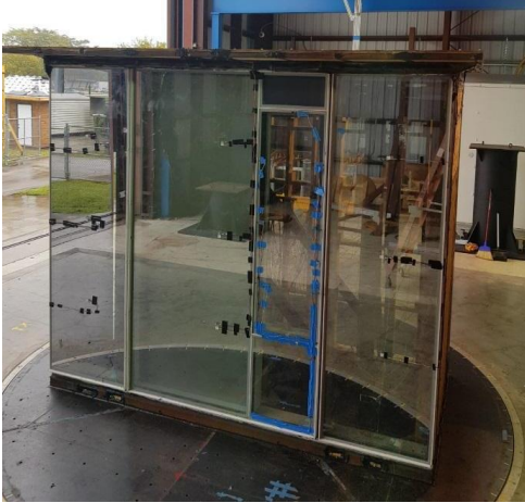
Figure 2.10: Curtainwall specimen on Turntable
