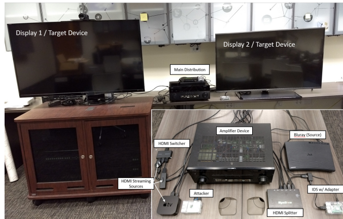
Figure 6.11: HDMI testbed, including two targeted displays, an attacker device, and the HDMI-Watch device within the same distribution.
