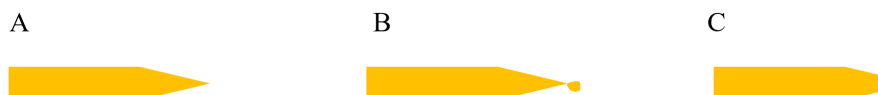
Figure 2-9 Sketch of the Au tip shape possibilities under an optical microscope. (A) Good. (B) Needs a second time etching, continue with step g). (C) Need to restart from the beginning, step a).
