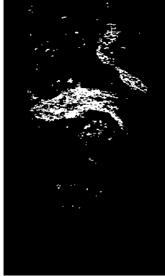
Figure (M3): Image filtering using Otsu's method and pixel area-based morphological filtering of small objects to isolate fish schools in each acoustic image. The processed image retains the main fish schools in the image and is ready for further processing to extract the boundary of the school of interest.
