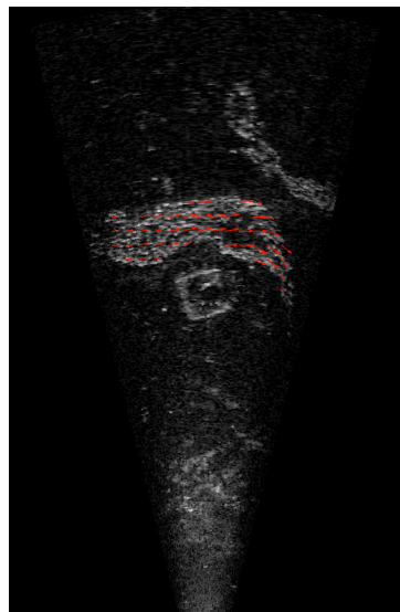
Figure (M6): Final detected school boundary with representative PIV velocity estimates used for analysis of schooling state. The optimized alpha shape school boundary was used to filter the PIV velocity field to include vectors located within the school, providing an accurate estimate of individual behavior within the school. Each school was tracked frame by frame via a Kalman filter over the course of the behavioral interaction.
