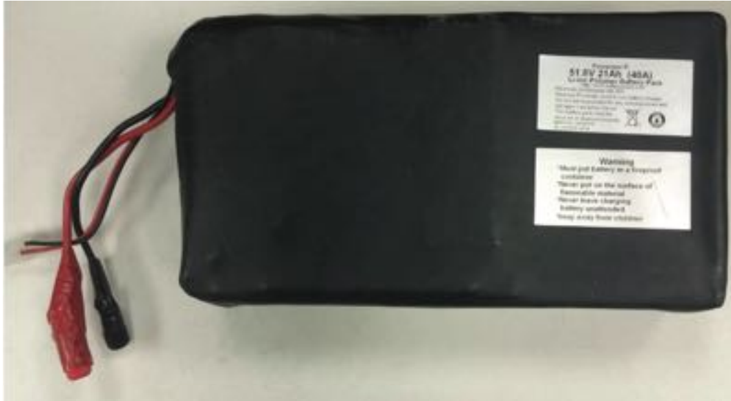
Figure 10.7 Lithium-ion battery bank module.
