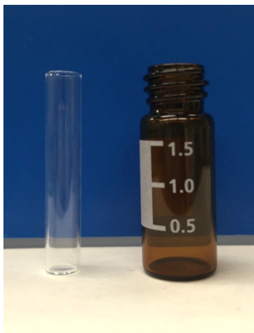
Figure 3.7: Vial insert and vials utilized for portable testing system
