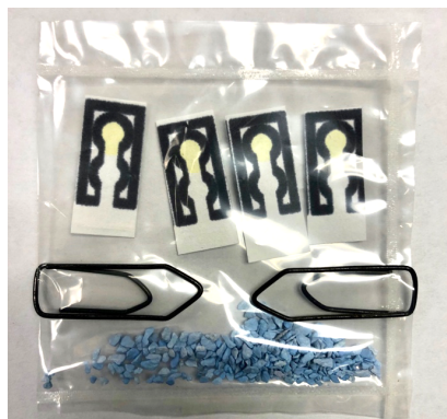
Figure 5.9: Single lane \mu PADs stored in sealed nylon bag with Drierite ®
