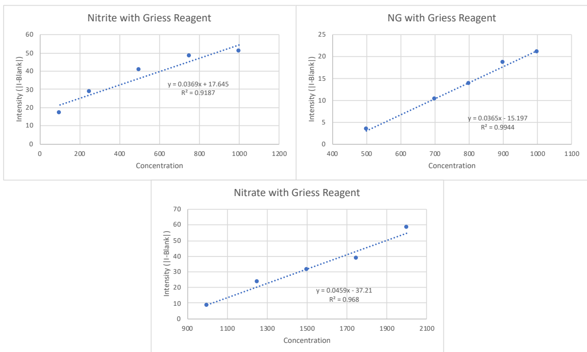
Figure 5.8: ImageJ linear fit plots of concentration ( \mu\text{g/mL} ) vs. color intensity for Griess Reagent
