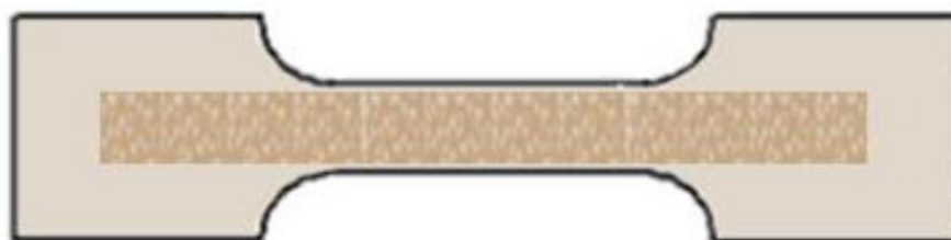
Figure 25: Schematic of SMP epoxy-GrF mold cast Composite
