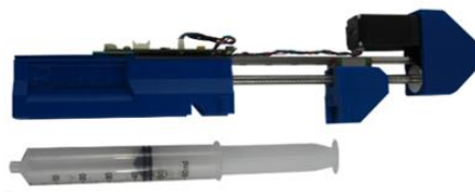
Figure 58: Print head syringe for low viscosity polymers respectively ( http://www.hyrel3d.com/core-suystems/system-30m )
