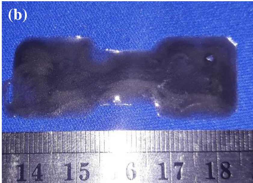
Figure 62: Images of 3D printed dog-bone shape sample placed under nearly cryogenic condition. a) SMP epoxy b) SMP epoxy-0.1 wt.% GNP
