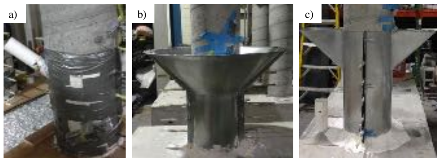
Figure 4- 6 Different forming used in this study to place UHPC.
