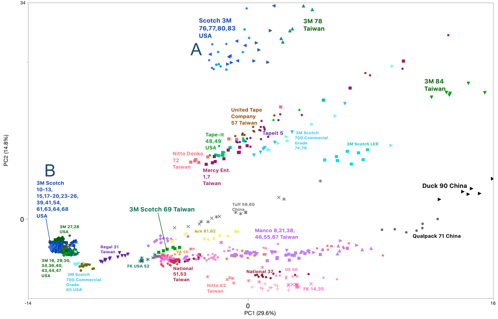
Figure 26 – PCA plot of the 90 electrical tapes selecting two principal components. A: Scotch 3M tapes containing barium, antimony, and magnesium. B: Scotch 3M containing high amounts of lead. 44
