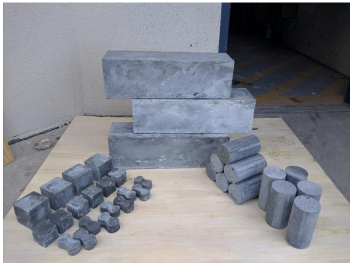
Figure 2-1 UHPC specimens after demolding.
