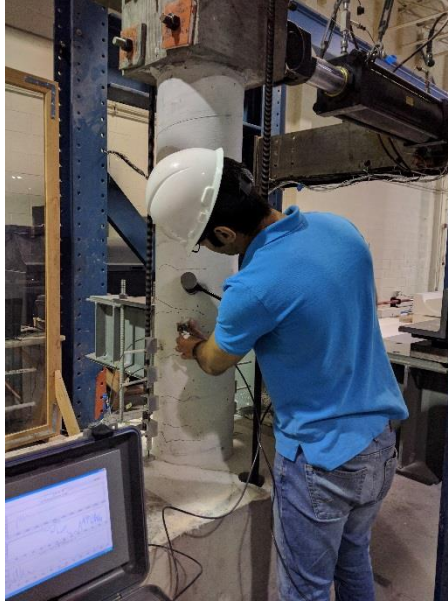
Figure 6-38 Measuring the mobility of the column.
