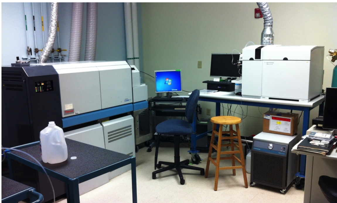
Figure 5. Thermo Element 2 HR-ICP-MS (left) and Agilent 7700x Q-ICP-MS (right) in the Trace Evidence Analysis Facility (TEAF) at FIU.
