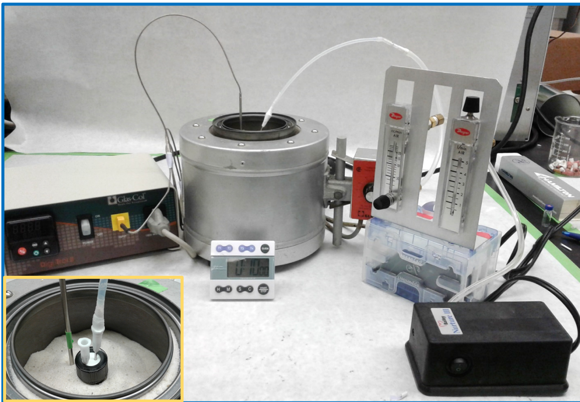
Figure 37. Sampling setup for headspace extraction of heroin samples using CMV.
