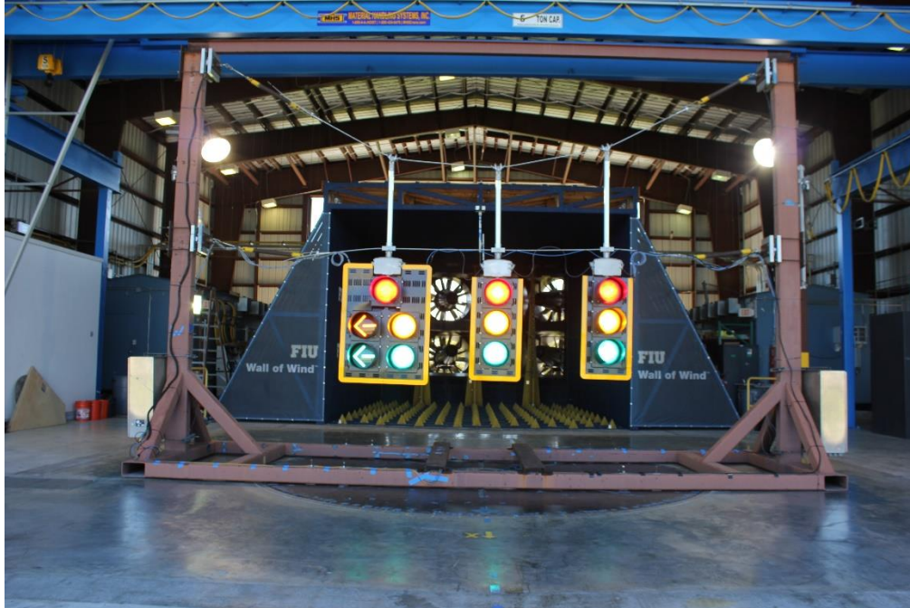
Figure 2-16 – Modified traffic light assembly (5% sag, 7 feet distance between catenary and messenger load cell, un-tensioned messenger wire)
