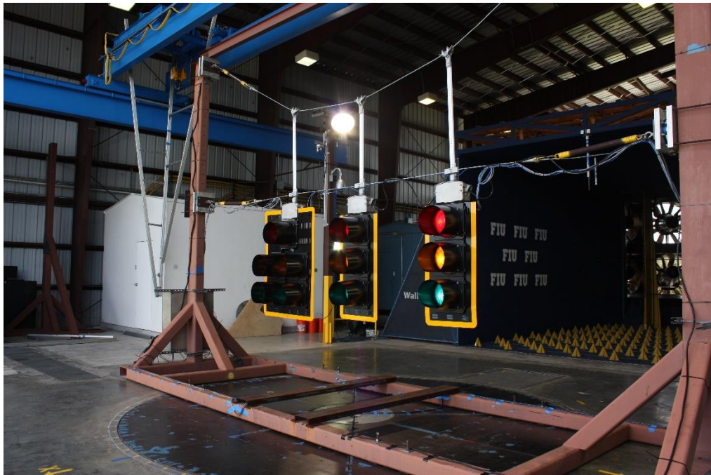
Figure 2-7 - Test rig with traffic lights assembly
