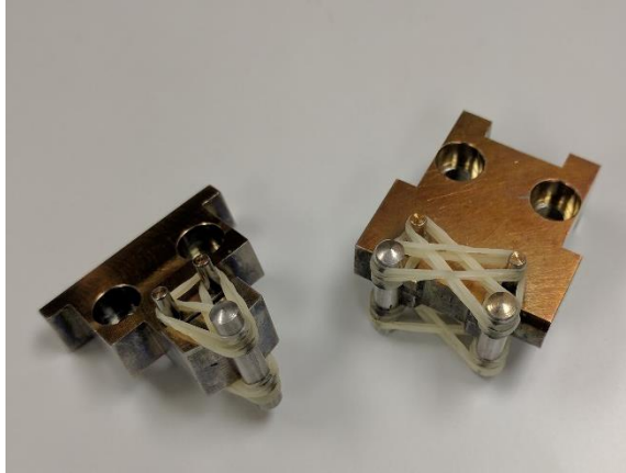
Figure 20. Micro-ENF fixtures configured in a three-point bend
