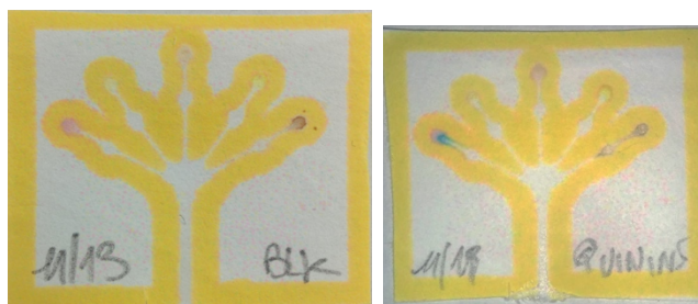
Figure 3.21 A demonstration of the \mu PAD developed to detect interferences: From left to right: Modified Scott's reagent channel, ninhydrin reagent channel, Fast blue B reagent channel, ferric chloride channel, permanganate/ molybdic acid channel. The results show a comparison of a blank chip (left) and a chip exposed to a sample of quinine (right), with a resulting change in the color of the modified Scott's reagent.
