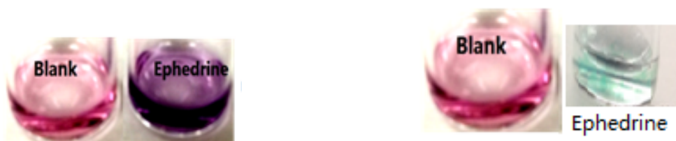
Figure 3.13. Color change observed for the modified Scott reagent. Left: ephedrine/methanol; Right: ephedrine/acetone. Ephedrine: 1mg/mL
