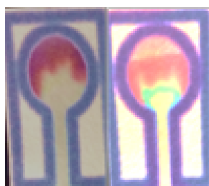
Figure 3.14. Color change observed for the modified Scott reagent on paper microfluidic device. Left: Blank test. Right: Cocaine test, cocaine 1mg/mL in 50% Acetone.
