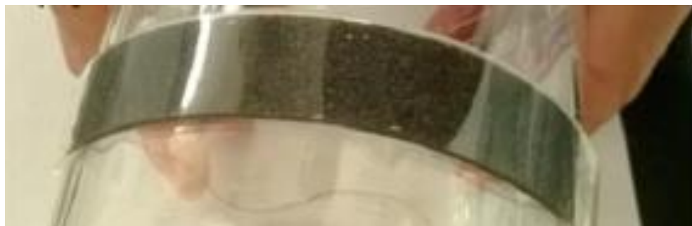
Fig. 2.13. Optical image of GrF-PDMS-PET composite bended over a beaker [89] .
