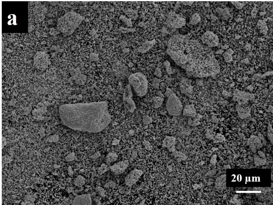
Figure 4.1: Agglomeration in as-received powders: (a) TaC, (b) HfC
