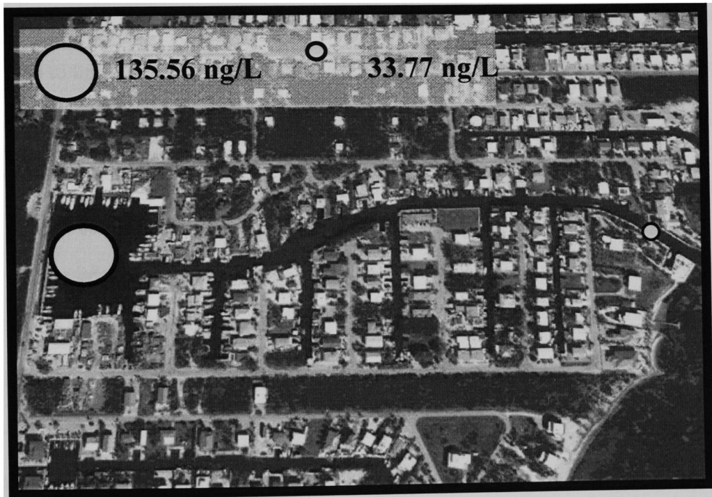
Figure 3.29. Satellite image of Lake Largo illustrating the diffusion/dispersion transport process from a distributed point source.
