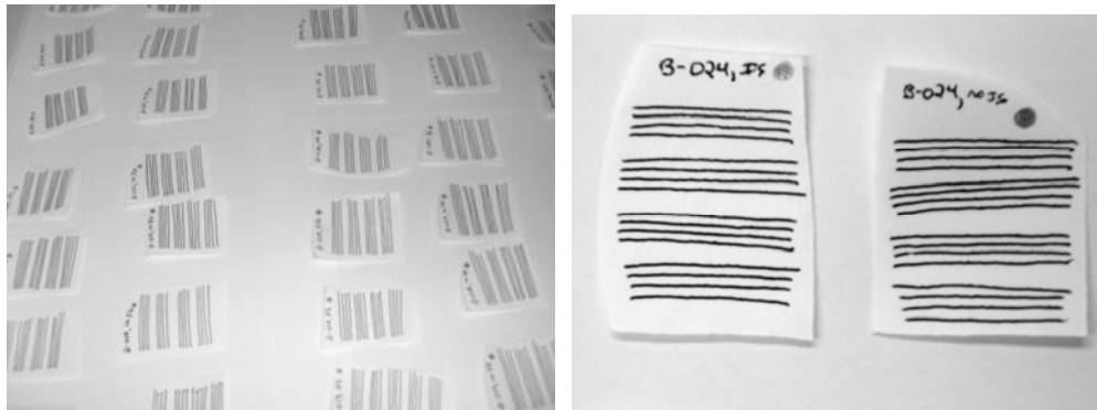
Figures 17(a) and 17(b). Photos of prepared black gel ink samples on Whatman 542 filter paper, collected pen set.
