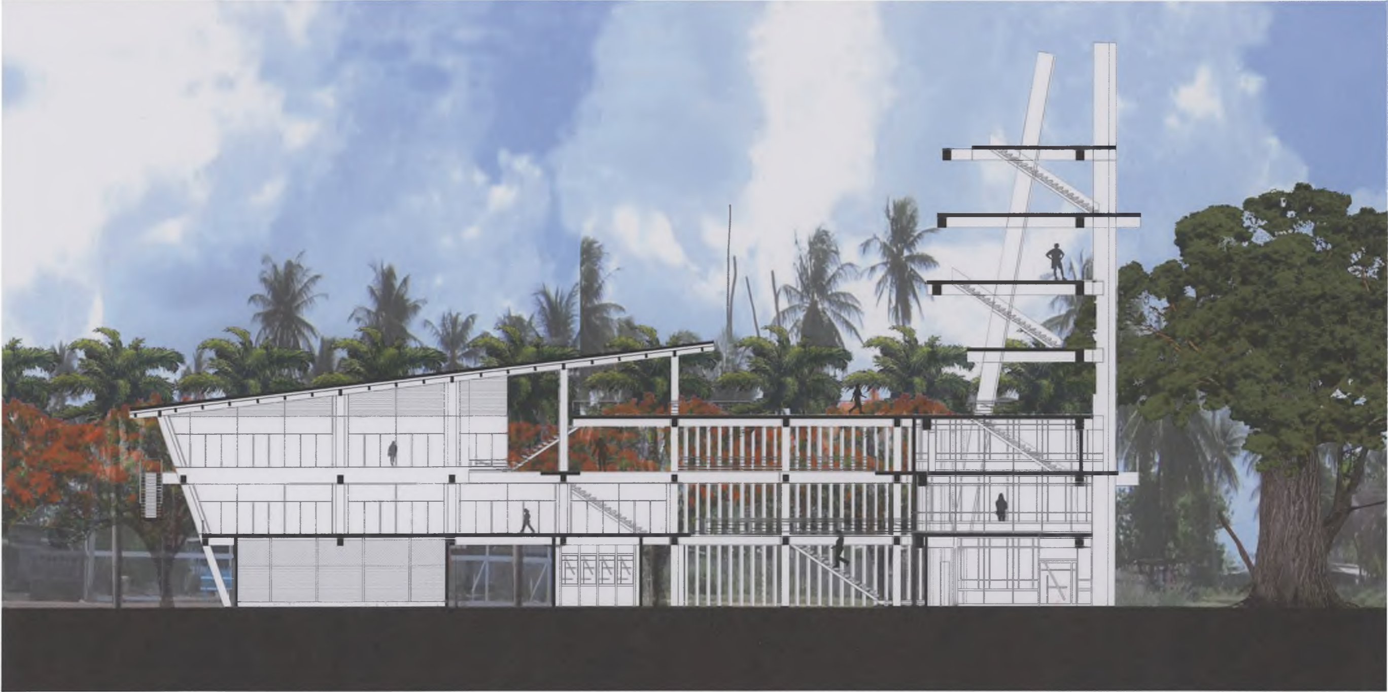
Figure 55: Section 01-east-west section through Library and Tower. Landscaping and structure combine to produce a vertical layering effect.
