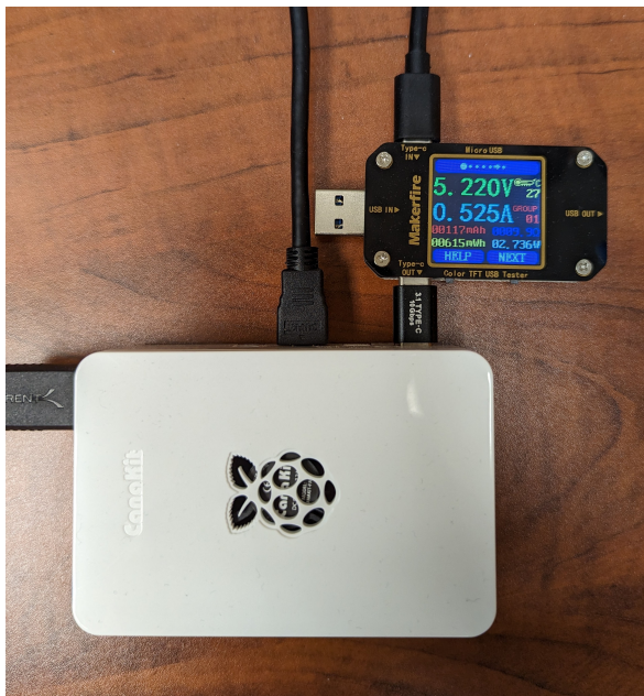
Figure 5.8: Our energy consumption setup for the Raspberry Pi using the MakerHawk USB Multimeter.
