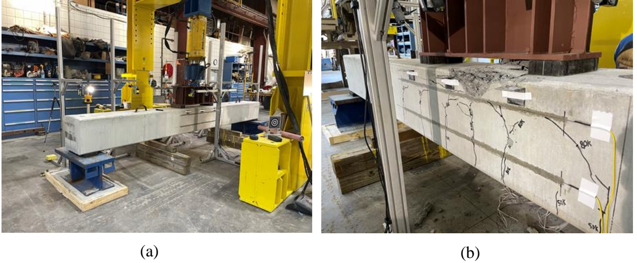
Figure 5.41: Flexure test pile setup
