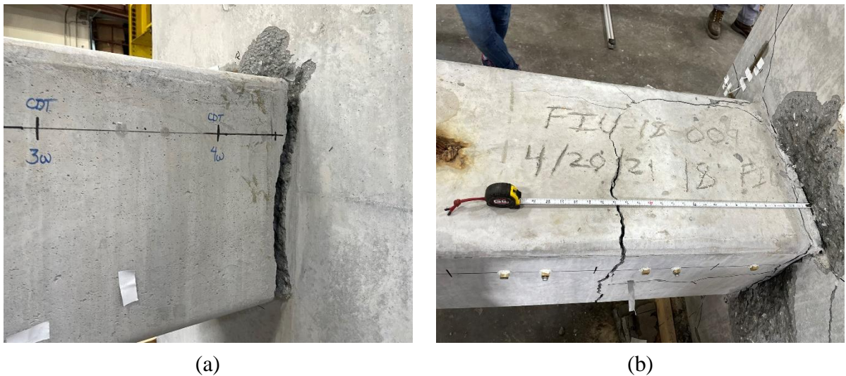
Figure 5.51: Photographs after failure for (a) SP-04 and (b) SP-03 with observed strand development failure
