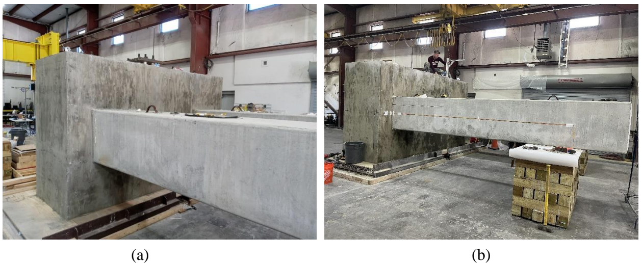
Figure 5.37: Finished 30-inch specimens (a) SP-09, (b) SP- 10
