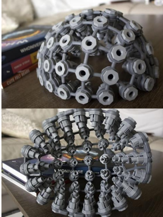
Figure 2.3. 3-D printed EEG cap
