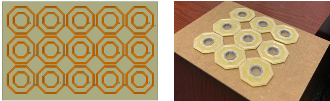
Figure 5.11 CAD model and experimental setup for powering resonator array.
