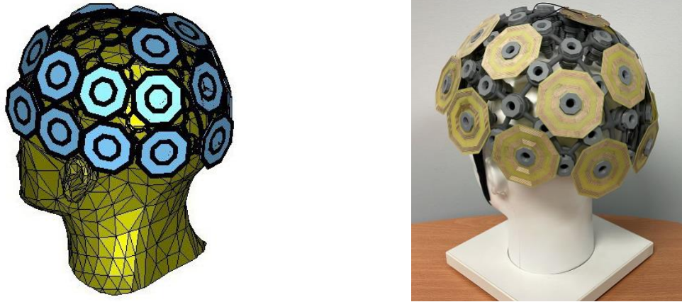
Figure 5.12 CAD model and Fabricated setup of power receiver resonator array (Front-end Rx array mounted on EEG head cap).
