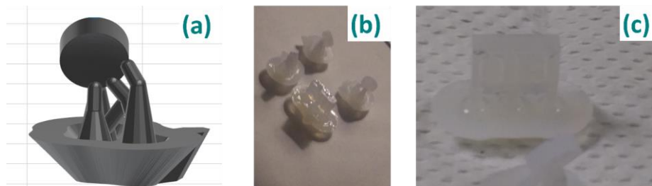
Figure A-2: (a) Computer aided model of a typical pellet utilized for printing the green bodies. (b) Printed green pellets and an exemplary structure on supports before calcination (c) An expanded view of the printed FIU green body structure still on the supports before calcination.
