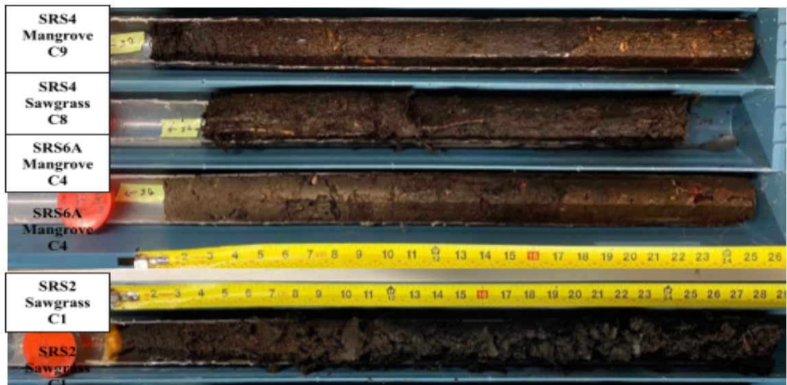
Figure 6. Four representative cores, SRS4 C9, SRS4 C8, SRS6A C4, and SRS2 C1 used for sediment analysis.
