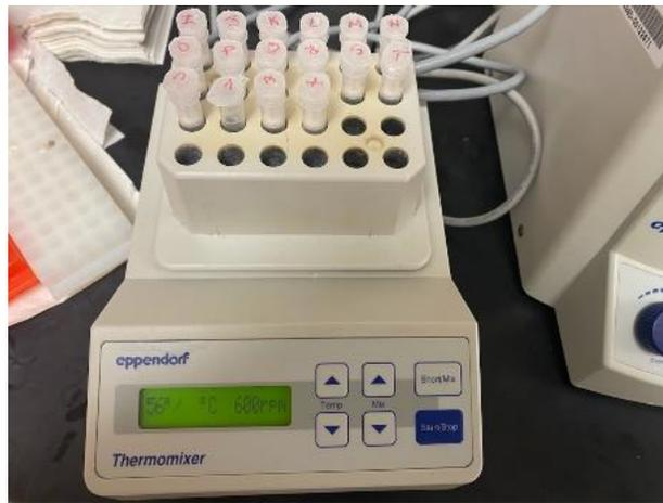
*Figure 45: Samples incubating in a heating block using an Eppendorf Thermomixer*
