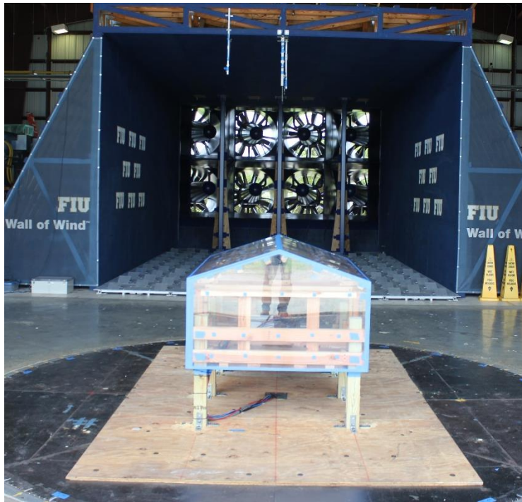
Figure 5.8 One-story 2.15 m elevated model inside WOW
