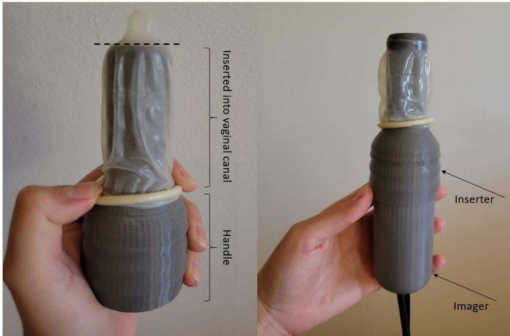
Figure 5.6 PPRIM device showing inserter and imager. The left image shows the inserter with a condom used to aid slide it into position. The dashed line shows where the condom is cut to not interfere with the image quality. The right image shows the device fully assembled including the inserter and imager.
