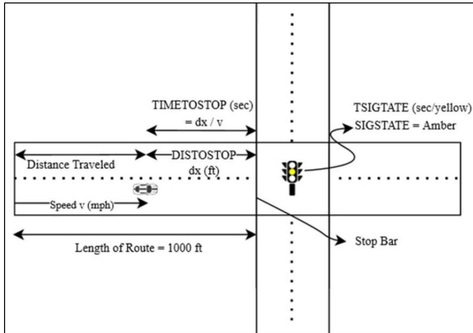
**Figure 3-7: Variables Affecting the Stop Decisions in the Simulation Model**
