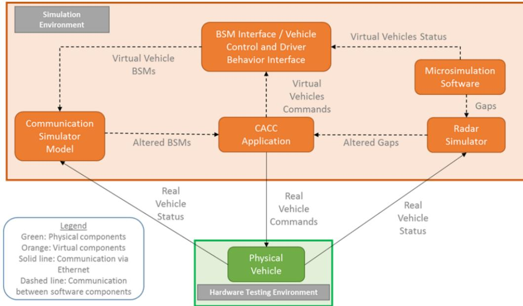
**Figure 2-2: CACC HIL Architecture (Ma et al., 2018)**
