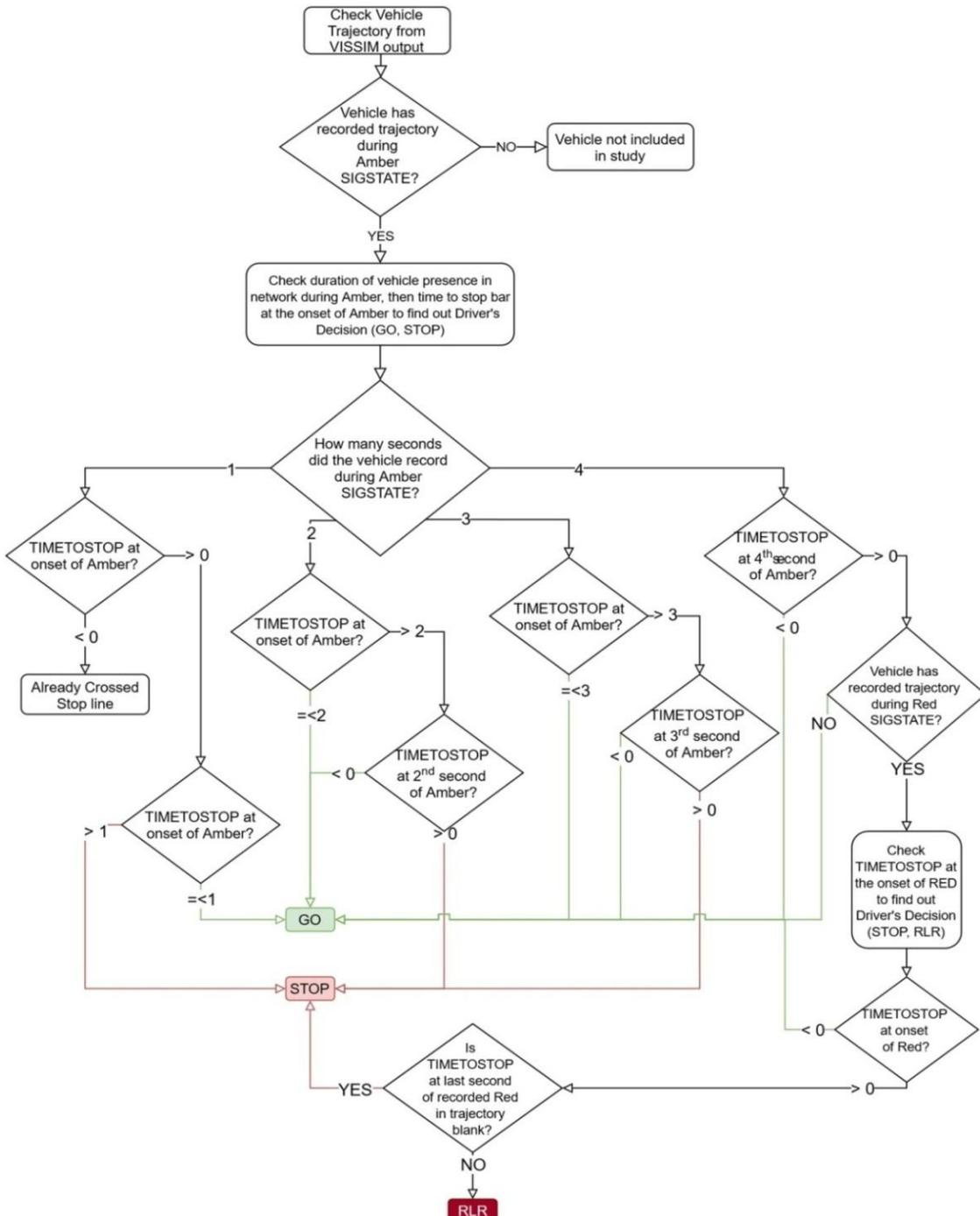
Figure 3-8: Vehicle Trajectories Analysis
