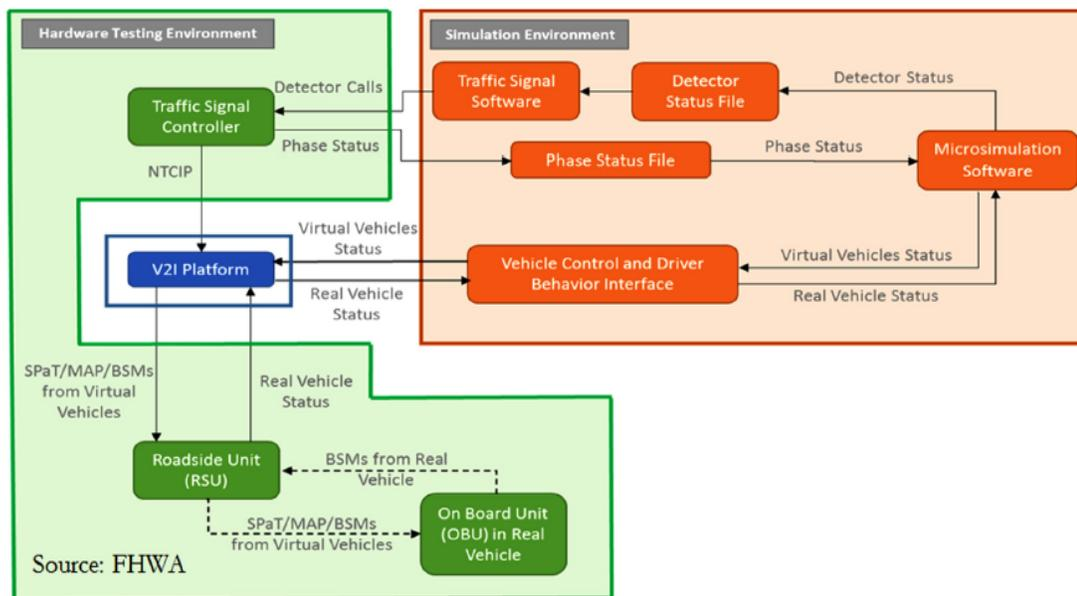
**Figure 2-3: Q-SIAD Architecture (Ma et al., 2018)**
