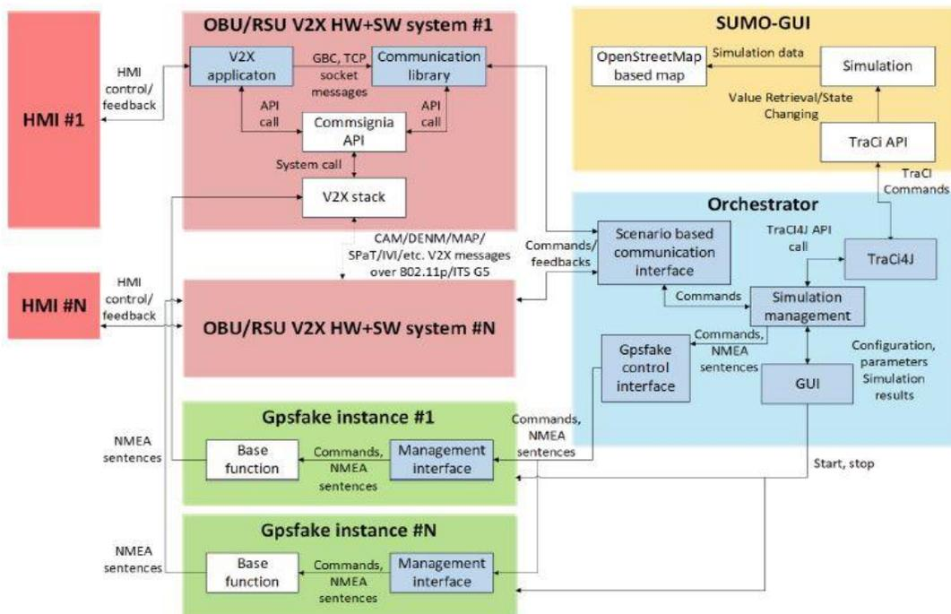
**Figure 2-5: HIL V2X Simulation Architecture (Szendrei et al., 2018)**
