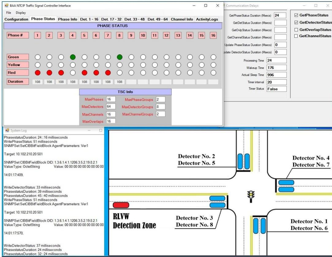
**Figure 3-4 HILS Middleware Interface and Detector Setup**
