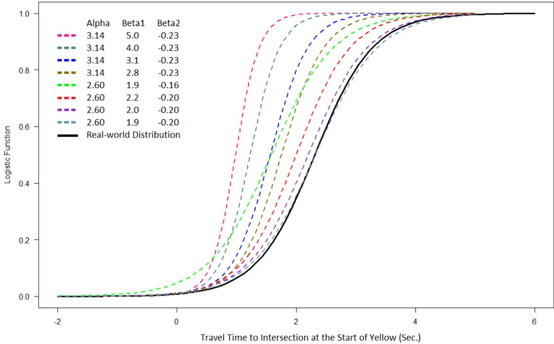
**Figure 4-1: Simulation versus Real-world Probability of Stopping**
