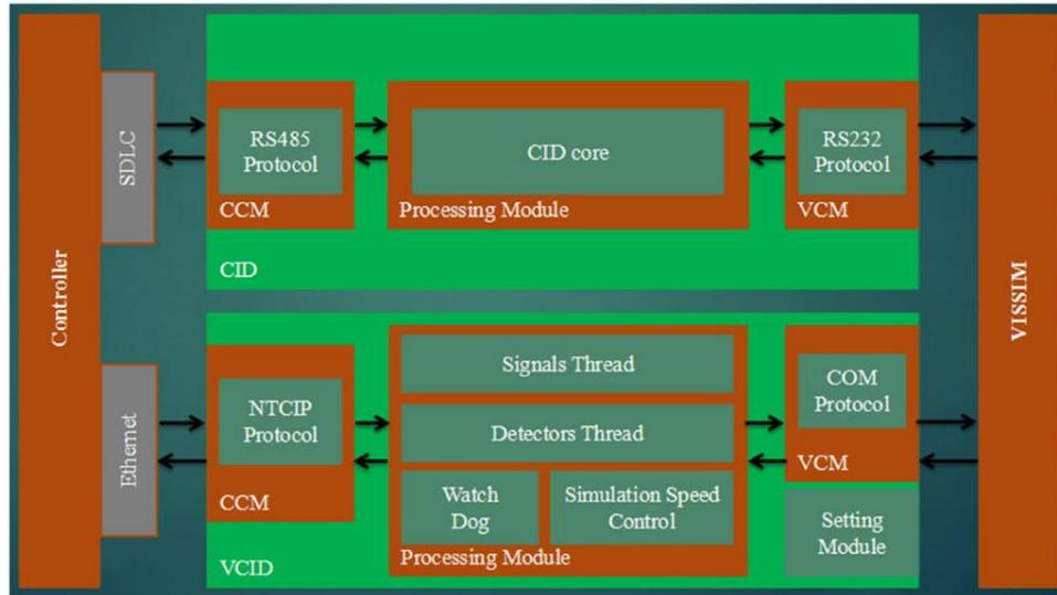
**Figure 2-1: CID and VCID Architecture (Wang et al., 2017)**
