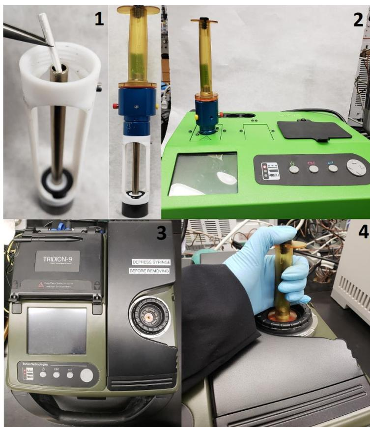
**Figure 17: Picture scheme of the CMV/NTD sampling protocol. CMV is inserted into the stainless-steel tube and sealed with the NT adapter (1). Holder with inserted needle trap is placed into SPS-3 for desorption method (2). Top view of the T9 portable GC-MS (3). Injection of the needle trap into the T9 after CMV desorption (4)**
