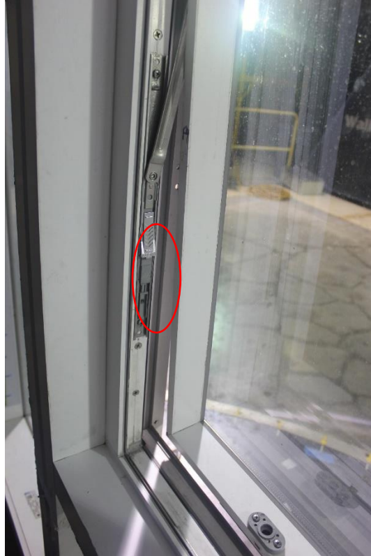
Figure 3.30: Yielded connection hinge
