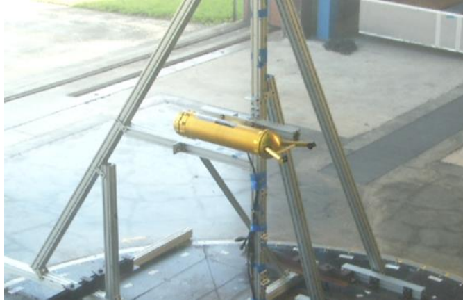
Figure 4.5: PIP at 0.91m. (6ft.) height located at turntable center
