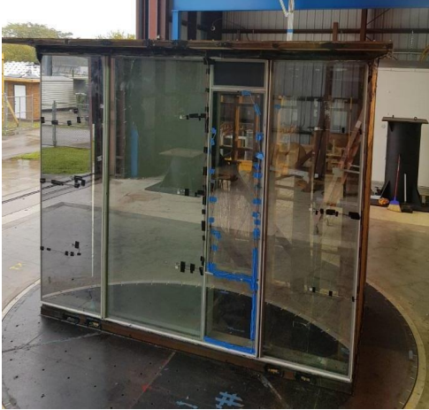
Figure 2.10: Curtainwall specimen on Turntable
