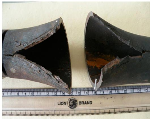
Figure 1.1: Failed section of a superheater tube [2].
