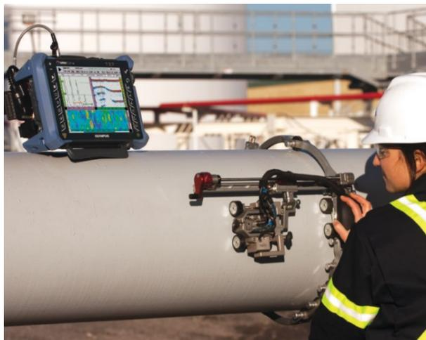
Figure 2.8: HydroFORM inspection tool [23].
