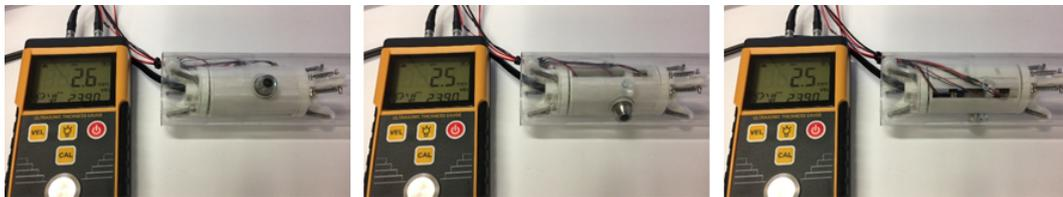
Figure 4.5: Measurements performed on the tube's inner surface.
