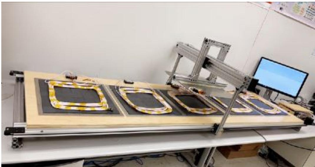
Figure 7.14: The experimental setup for dynamic IPT system which is built based on "POS-6" design values
