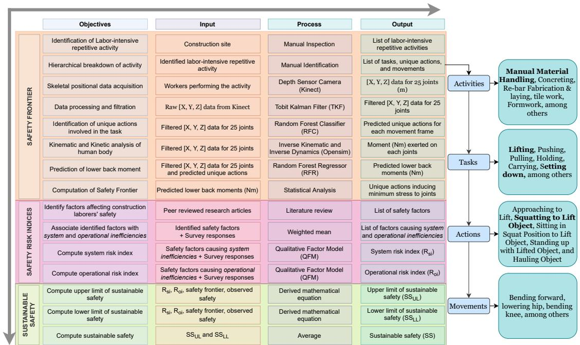
Fig. 6.1. Methodology to compute *safety frontier* and *sustainable safety*
