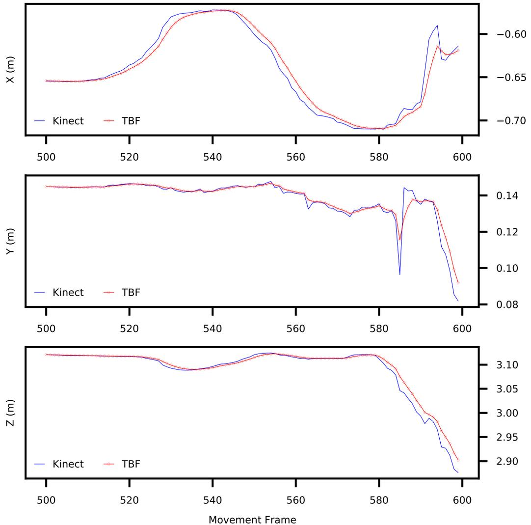
**Fig. 6.4.** Spatial coordinates of spine base obtained from *Kinect* before and after applying TKF
