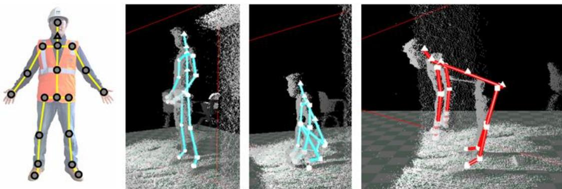
**Fig. 4.4.** (Left to right) Joints in the human body, joints detected by *Kinect* camera, good lifting posture, bad lifting posture in red
