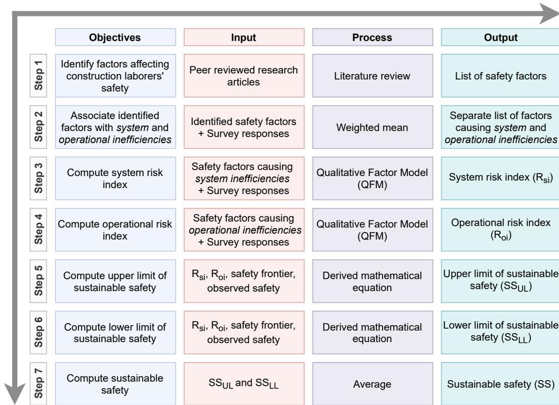
Fig. 5.2. Methodology to compute *system* and *operational inefficiencies*
