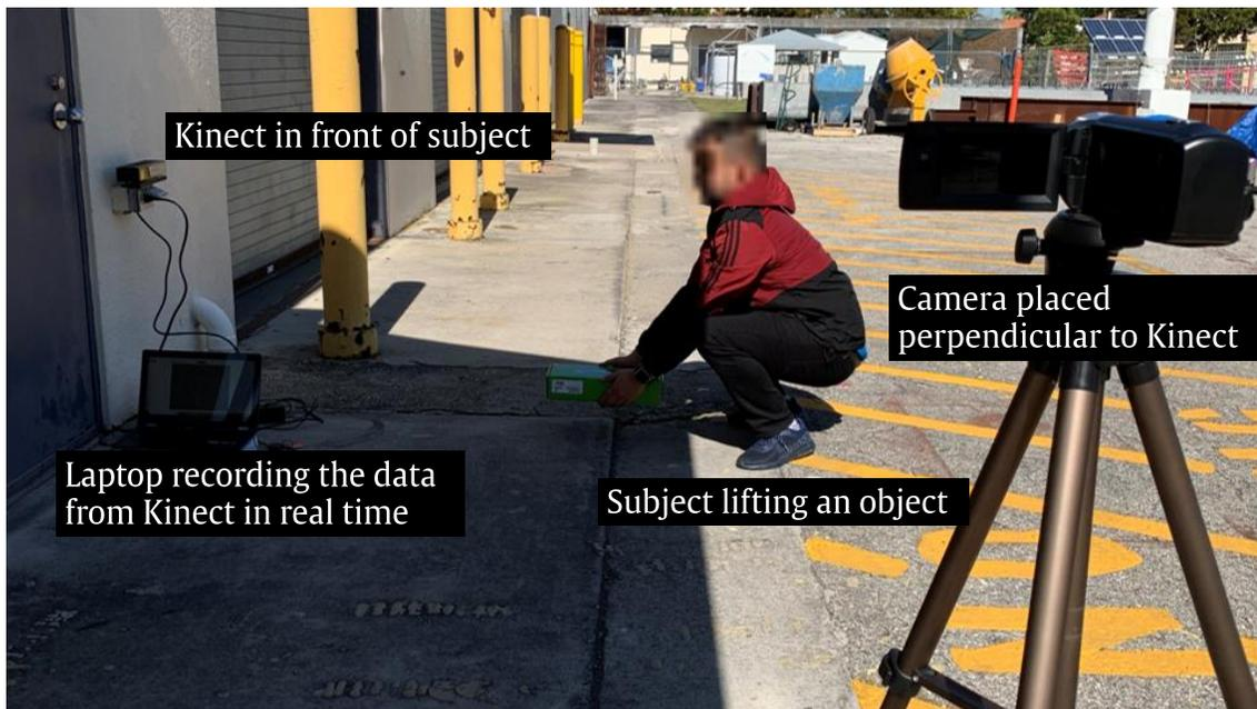
**Fig. 4.5.** Typical equipment setup for data collection
