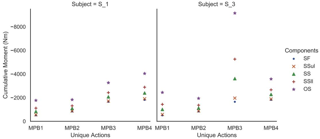
**Fig. 6.12.** Cumulative moment for four unique actions of the metal plate bending for different safety components
