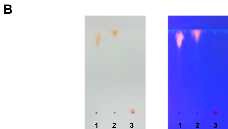
Figure 4.2. (A) An experimental procedure to synthesize and purify DNR-GTP, DNR-dGTP, DOX-GTP, and DOX-dGTP conjugates in 10 mM sodium borate buffer pH 8.2. (B) Thin layer chromatography (TLC) of DNR (lane 1), DNR in the presence of 2% HCHO (lane 2), the DNR-GTP conjugate (lane 3). Samples were spotted on Silica Gel 60 F 254 and developed with a mobile phase of chloroform: methanol: acetic acid = 16:4:1 (v/v). After the development, the TLC plates were photographed under visible (left panel) and UV light (right panel).
