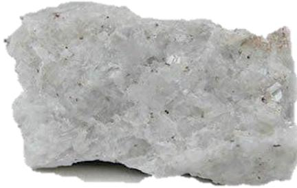
Figure 3: Specimen of granular dolomite from Thornwood, New York.
