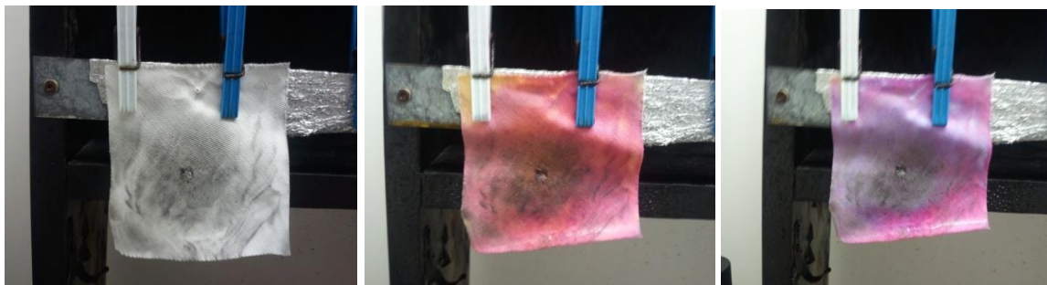
Figure 1.2: Pictures of the sodium rhodizonate test for Pb in action: The left picture shows a square of white denim that was shot by a Glock-17 9mm pistol at a distance of 6 inches. The middle picture shows that same cloth after 3 sprays from a spray bottle containing a concentrated aqueous sodium rhodizonate solution and a 0.1 M pH 2.8 sodium bitartrate/tartaric acid buffer in aqueous solution. The Pb from the gunpowder turns a deep red color. The right picture shows that same cloth after 3 sprays of 5% HCl. This confirmatory step makes the Pb, and only the Pb, turn a blue-purple color (pictures taken by the author J. A. Silverman).
