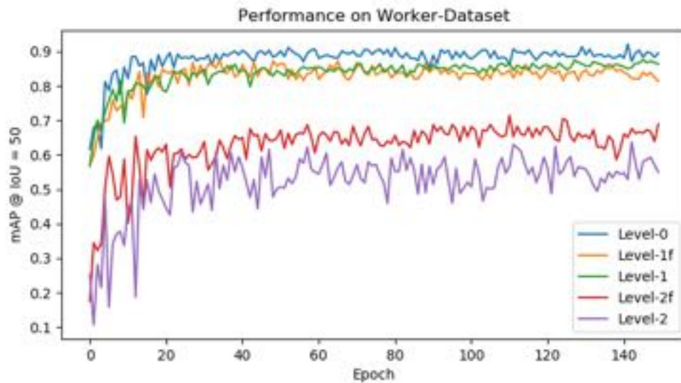
Figure 4.28: Performance on worker dataset. Compared with the level-0 data, the level-1 and level-1f shows competitive effect in training.
