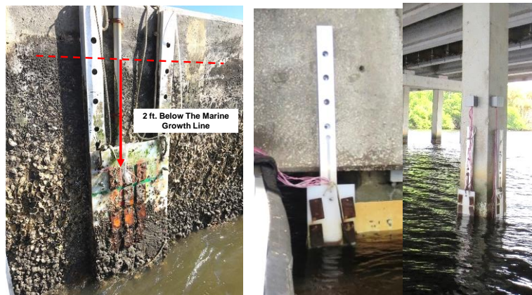
Figure 5.3. Typical Outdoor Exposure Test Rack at Three Site
