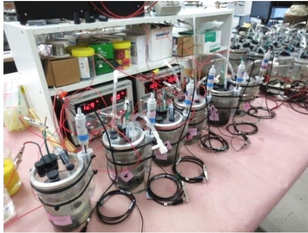
Figure 6.1. Test Setup B test cells under cathodic polarization
